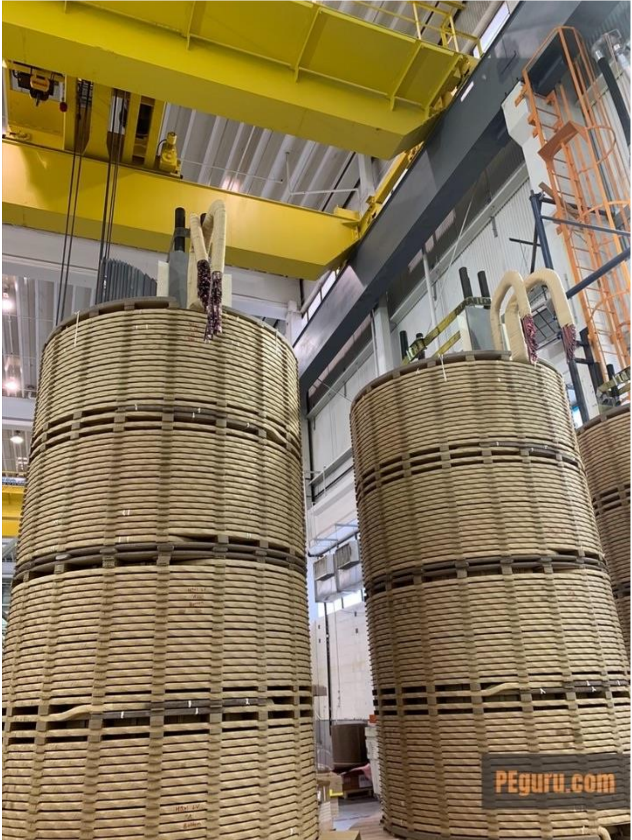
Low voltage winding on laminated sheets of core metal
